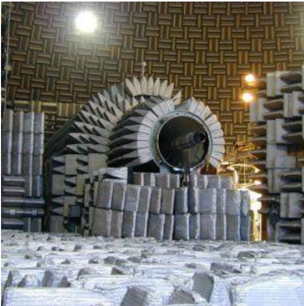
Nozzle Acoustic Test Rig (NATR) in the Aero-Acoustic Propulsion Laboratory (AAPL).
